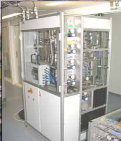
Test Rig with Reformer for SOFC Application
