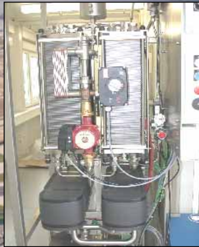
Test Rig with Integrated PEM Fuel Cell
