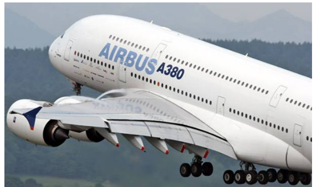
Fig 1: Airbus A380 in high-lift configuration
