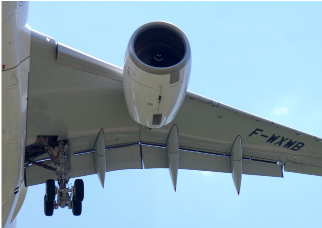
Fig.12: A350XWB Adaptive Dropped Hinge Flap in flight in full deflected setting
