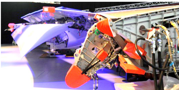
Fig.9: Adaptive Dropped Hinge Flap: inboard flap support station (flap not assembled), deflected outer flap and deployed spoilers
