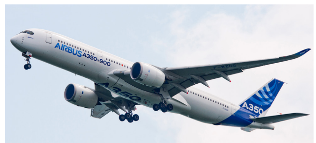
Fig.4: The A350XWB in high-lift configuration
