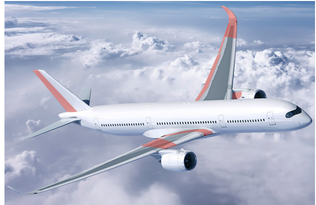
Fig 16: Local active separation control – potential areas of application on future transport aircraft configurations (in red)
